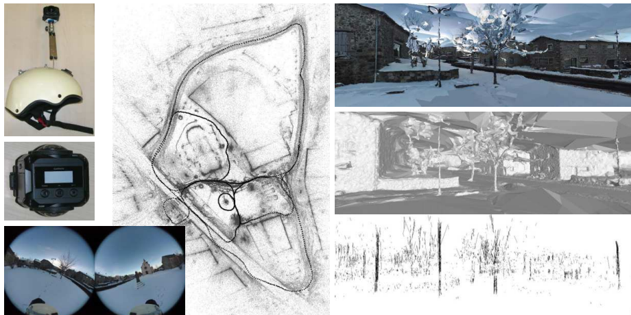
Fig. 2. Left: the helmet-held Garmin Virb 360 camera and one keyframe. Middle: a top view of the SfM point cloud and the camera trajectory. Right: A view of the final surface reconstructed by step 6b and the vertical edges (the set E' ) that we use.
