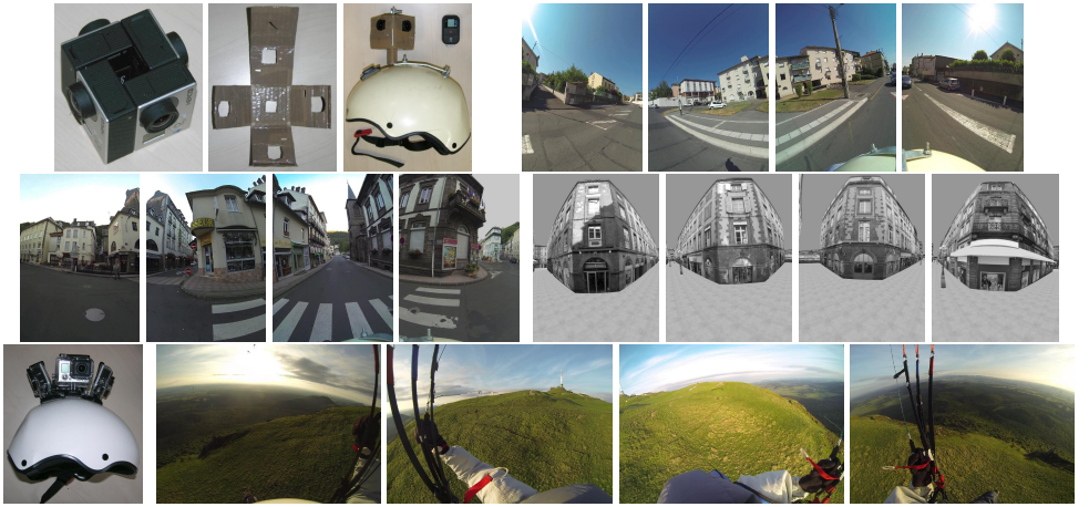
Figure 1: Two multi-cameras formed by four GoPro Hero3 cameras and images taken at a viewpoint for every dataset. Top and middle: the cameras are enclosed in a cardboard (for small baseline). Bottom: the housings provided with the cameras are used.
