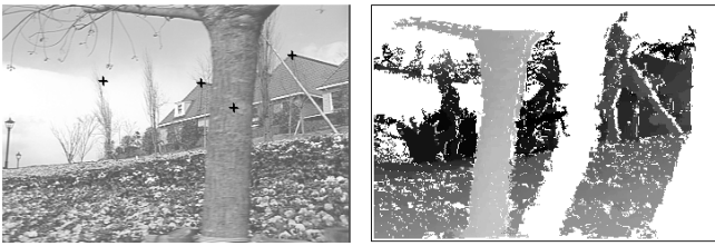
Figure 3. Left: Four manually selected seed matches. Right: the resulting disparity map.
