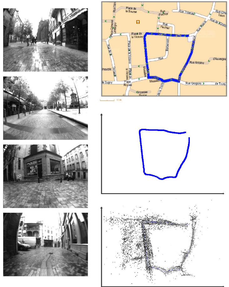
Figure 5. The long urban sequence a) left: some frames from the sequence, b) right: a map of the city with the trajectory in blue, the reconstruction result (trajectory and 18.403 3D points).
