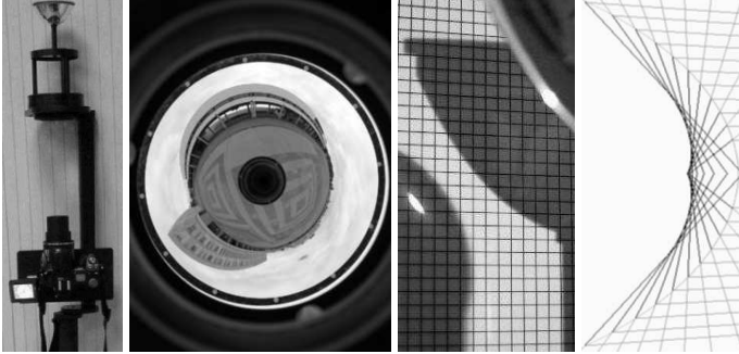
Figure 5: From left to right: the Kaidan “360 One VR” mirror with the Nikon Coolpix 8700 camera (mounted on a monopod), a panoramic image (the view field is 360^\circ horizontally and about 50^\circ above and below the horizontal plane), the mirror shadow for profile estimation, and the mirror caustic for \mathcal{P} = 50cm .
