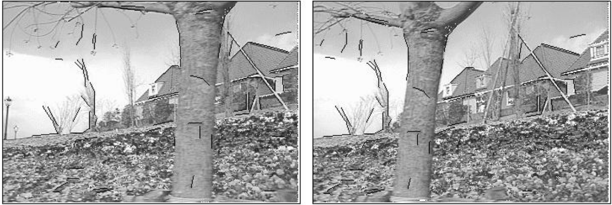
Figure 10: Detection of line segments as edge constraints by deduction from the disparity map. The corresponding line segments are displayed in black.
