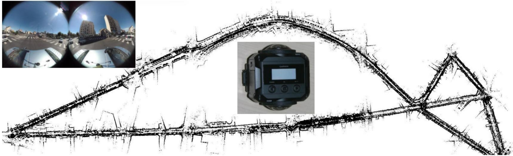
Fig. 2. One keyframe, the Garmin Virb 360 camera, and a bottom view of the vertices of T .
